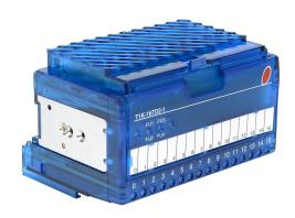
Terminator discrete output module, 16-point, 12-24 VDC, sourcing, 4 common(s), 4 point(s) per common, 1A/point, 4A/common. Requires T1K-16B or T1K-16B-1 terminal base.
