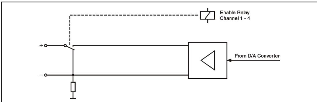
Figure 148: AM050 output circuit diagram
