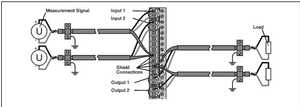
Figure 145: AM050 signal cable connection
