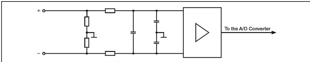
Figure 147: AM050 input circuit diagram
