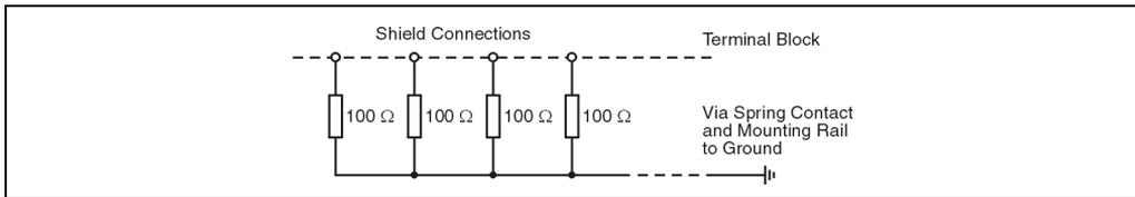
Figure 146: AM050 shielded connection
