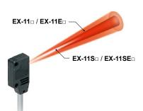
Possible to sense a minute object less than  $\emptyset 0.5 \text{ mm } \emptyset 0.039 \text{ in with}$ no slit.
