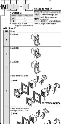
Some options are unavailable depending on the piping specifications. Refer to "Combination of piping specifications with option 1 and part numbers of options".
