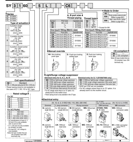
Note 1) The DIN terminal of the SY3000 series cannot be mounted on a standard manifold. For details, refer to page 639. Note 2) Enter the cable length symbols in ... Please be sure to fill in the blank referring to page 642. Note 3) When ordering single unit of the cassette type solenoid valve, the bushing assembly is included.
